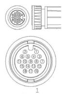
Connector 2 - Radar NMEA/Communications pin assignments
